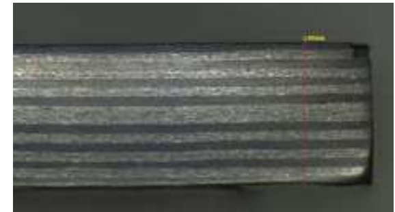
Out of autoclave consolidation micro cut
