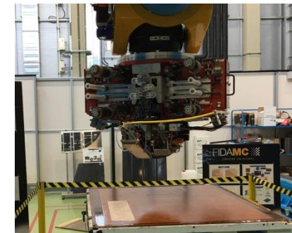
MULTI-TOW HEAD CONCEPT DEVELOPED WITH MTORRES
