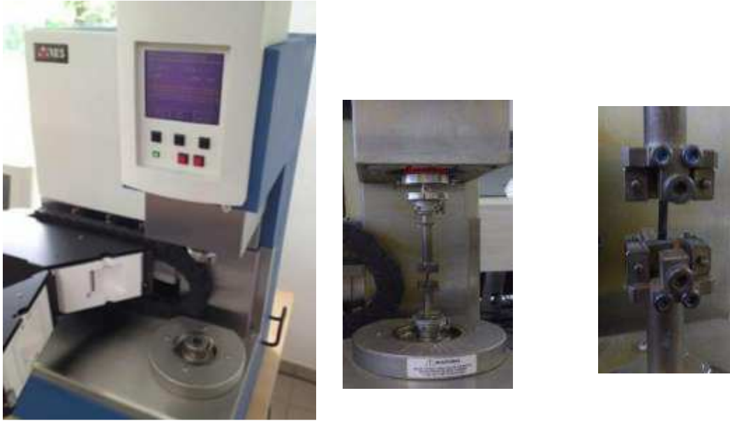
Figure 6: Dynamic mechanical analysis in torsion at CRT
