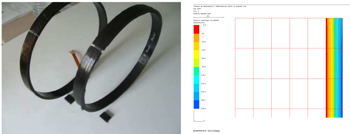
Figure 5: Evolution of residual strain gradient on composite after curing on [90]_{20} lay up
