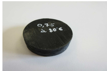
Lay-up (0/90/0/90/0)8. Targeted thickness 10mm.
