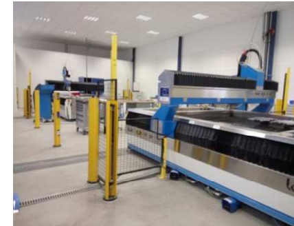
Fully automatized Water jet cutting Pressure > 4000 bar • 6 x 2 m • 4 x 2 m
