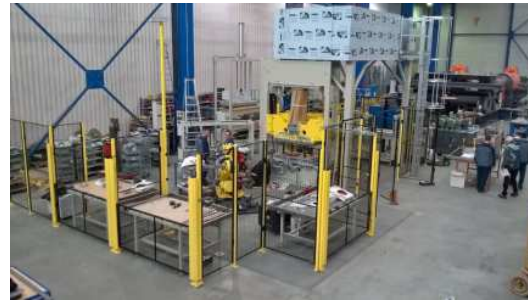
Fully automatized Thermo stamping 450° 200 Tonnes
