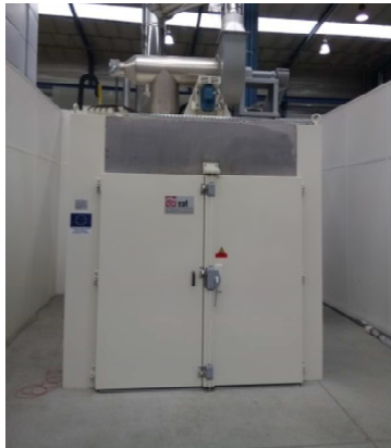
Consolidation Out of Autoclave 450° 10 m 3
