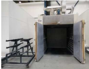
Consolidation Out of Autoclave 450° 10 m 3
