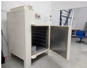
Consolidation Out of Autoclave 450° 1 m 3
