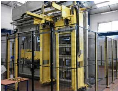
Thermo welding 450° 175 Tonnes
