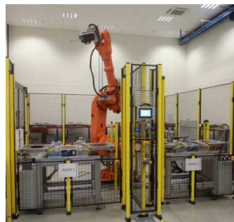
Automatized Induction Welding Robot 6 axis Accuracy 0,3 mm
