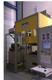
Thermo welding 350° 15 Tonnes
