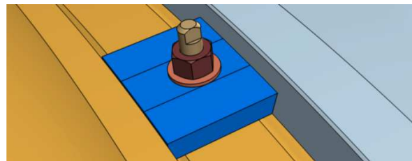
Figure 2: Axial stoppers principle
