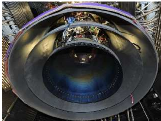
Figure 10: Full Nozzle Extension NE1 unlatched in the P 4.1 test cell
