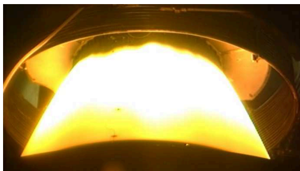
Figure 5: S1 A cone in P4.1 during M2 campaign firing - Heating phase
