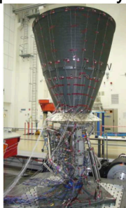
Figure 15: Nozzle Extension NEQ at IABG during EDQ dynamic test campaign
