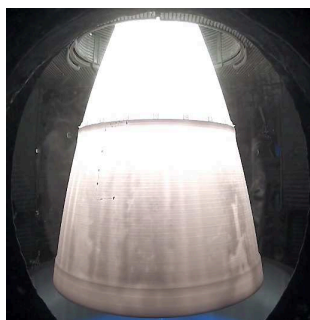
Figure 14: Full Nozzle Extension NE3 in P4.1 during M6 campaign firing
