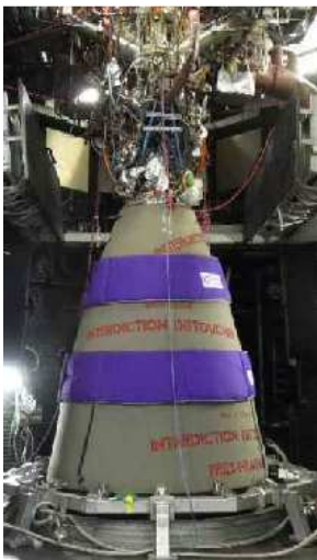
Figure 11: Full Nozzle Extension NE1 in P4.1 before firing
