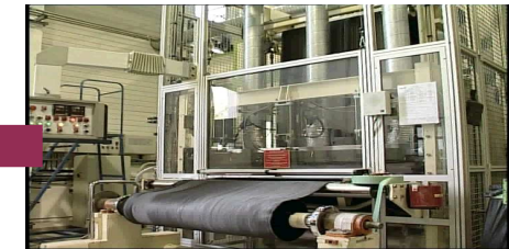
Impregnation with phenolic resin
