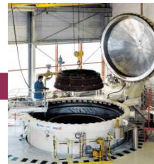
Autoclave resin curing
