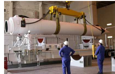
Orbital ATK employees loading a GEM 80 motor at Cape Canaveral Air Force Station onto the TTT (Traveling Trunnion Trailer) in preparation for ULA transportation to the pad for Delta IV mating.
